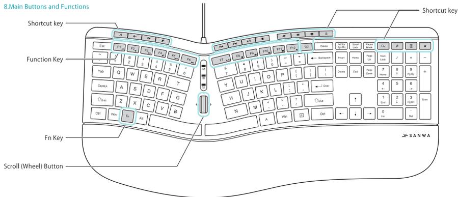
Press the function key or press the shortcut key at the top while holding down the Fn key to use the following functions.
